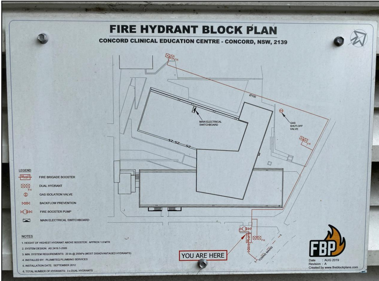
Figure 9 - Fire Hydrant Block Plan, building 26
