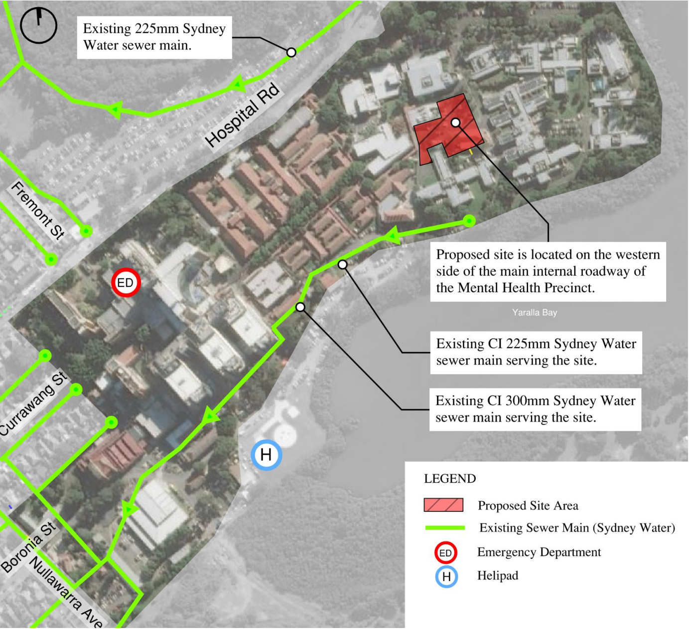
Figure 5 – Sewer drainage authority infrastructure serving the site
